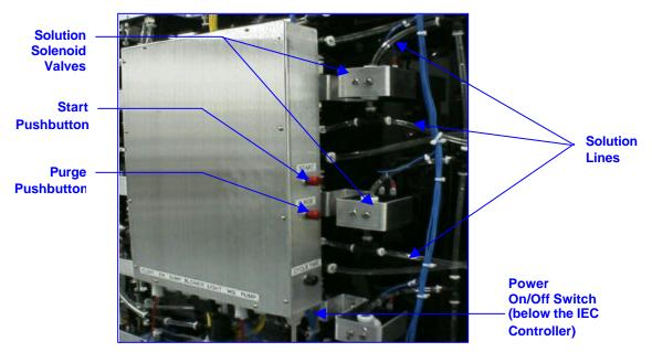
Figure 12: Location of Purge Pushbutton, Solution Lines, & Solution Solenoid Valves
