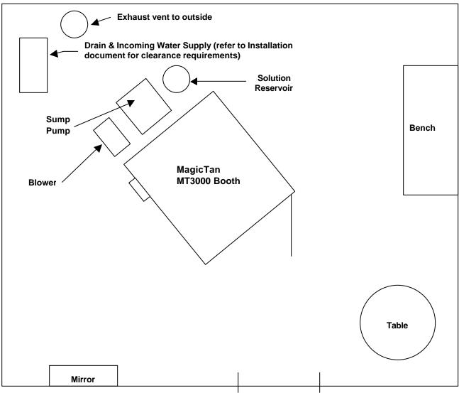
Figure 3: MT3000 Typical System Arrangement
