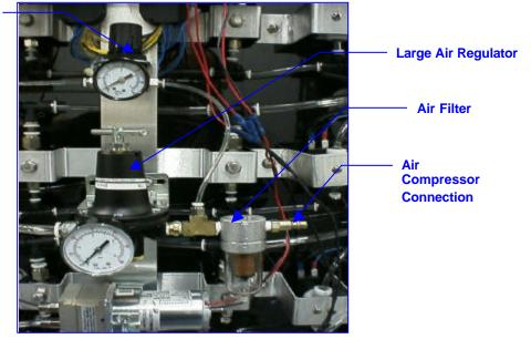
Figure 8: Location of Fluid/Air Controls (A)
