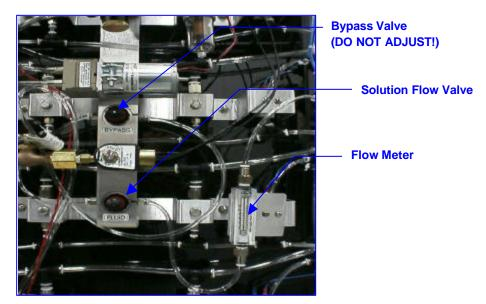
Figure 9: Location of Air/Fluid Controls (B)
